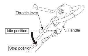
**Figure 19. Throttle Lever (Stop Position)**
